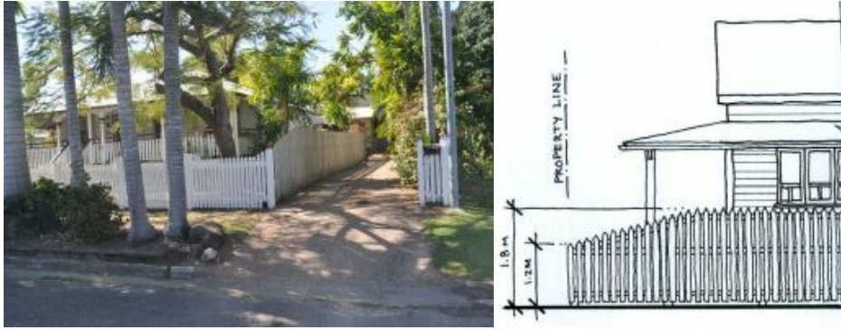
Figure SC6.2.5.1 Illustrates access strip fencing tapered from the front façade of the building to the street boundary (measurements are provided only as an example)
